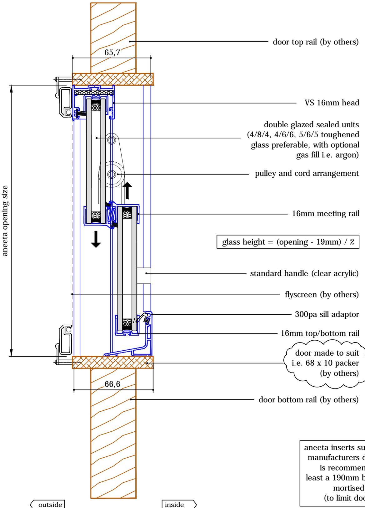
aneeta inserts suit a variety of manufacturers door types. It is recommended to use at least a 190mm bottom rail and mortised corner joints. (to limit door movement)
