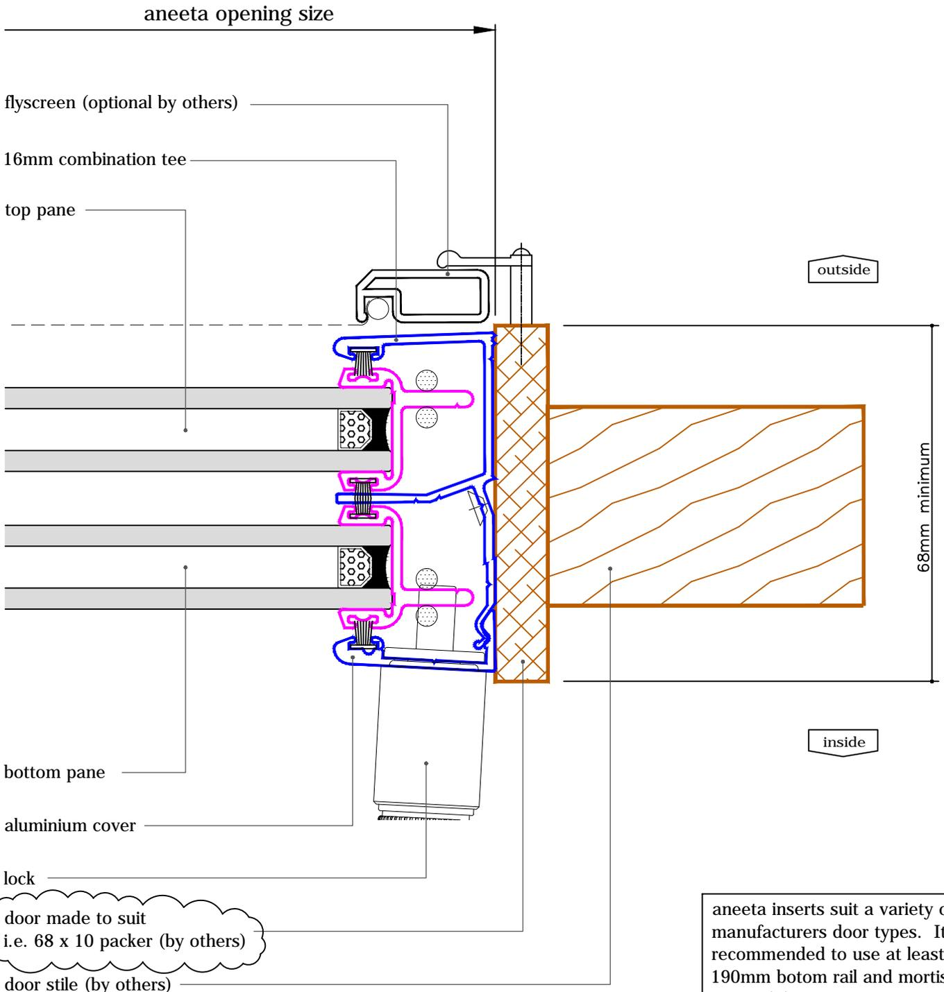
aneeta inserts suit a variety of manufacturers door types. It is recommended to use at least a 190mm bottom rail and mortised corner joints. (to limit door movement)
